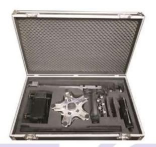
Box 1: Consists of Main Machine Assembly along with Mounting plate for wedges, Main Machine holder with Pressure controller, Arms, Bottom Plate Vice, Holding Plate, Electric / Pneumatic Motor
