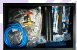
Box 2: Consists of Abrasive Papers, FRL, Pneumatic Motor, Pen Knife, Measuring Tape, Flash Light, Spanner Set, Allen Key Set, Adjustable wrench and other consumables.
