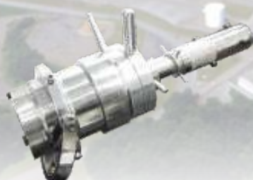
Seal Face Lapping Machine mounted on END FITTING
