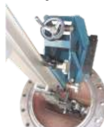
View from bonnet FG machine assembled on valve seat 10" x 300#
